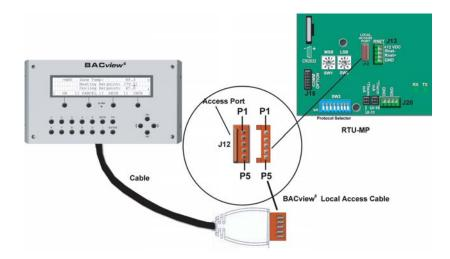
Fig. 68 - BACview<sup>6</sup> Handheld Connections
